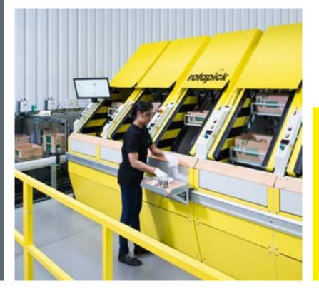
Three rotapick highperformance picking systems achieve up to 1 000 picks per hour; with these units, the warehouse movements are significantly reduced.
