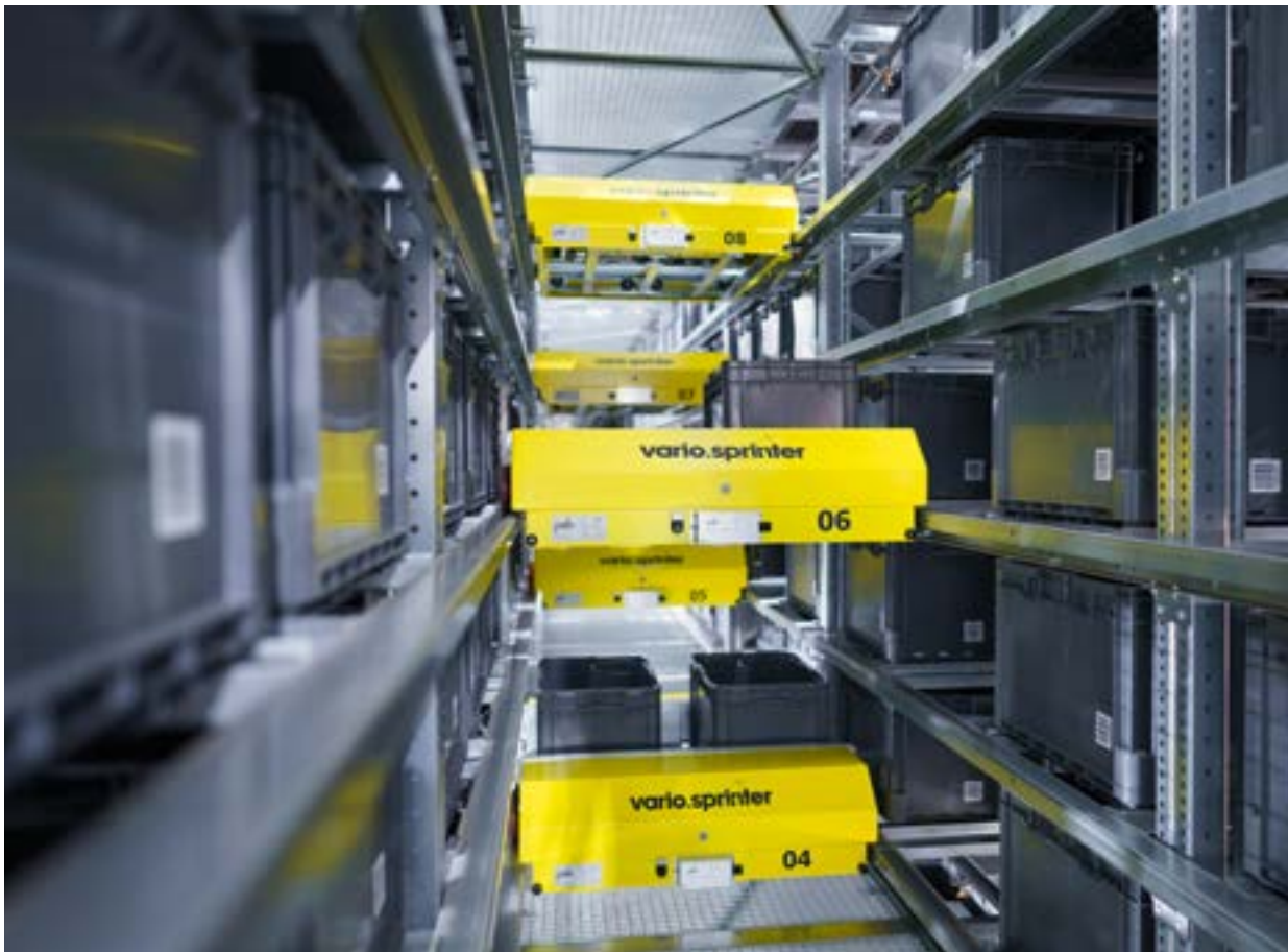
↑ Multi Access Warehouse: dynamic and easily expandable
